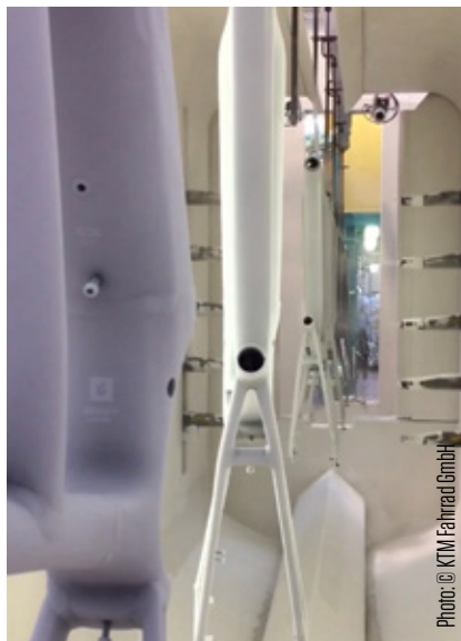
THE PRIMER AND FINISH ARE APPLIED TO THE BICYCLE FRAMES IN THE FULLY AUTOMATED POWDER COATING LINE.
