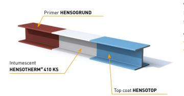
With a fire resistance time of R30–R60, the fire protection system HENSOTHERM<sup>®</sup> 410 KS is suitable for the following applications on steel structures:
